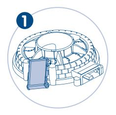
Fit the peg on one side of the cargo tray into the hole in the tower base. Press and "snap" the peg on the opposite side of the tray into the other hole in the base.
